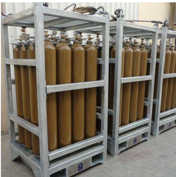
Oxygen cylinders secured in cage
