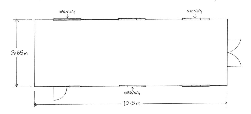
SCALE 1:50 PAPER SIZE A4 6 WINDOWS { 5 AT 1450mm × 660mm WOOD FRAME, GLAZED { 1 AT 507mm × 660mm
