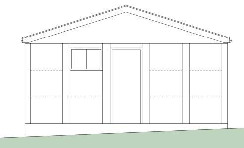
Scout Hut Building Profiled sheet roof covering Gable spandrel panel in wood stain plywood.
