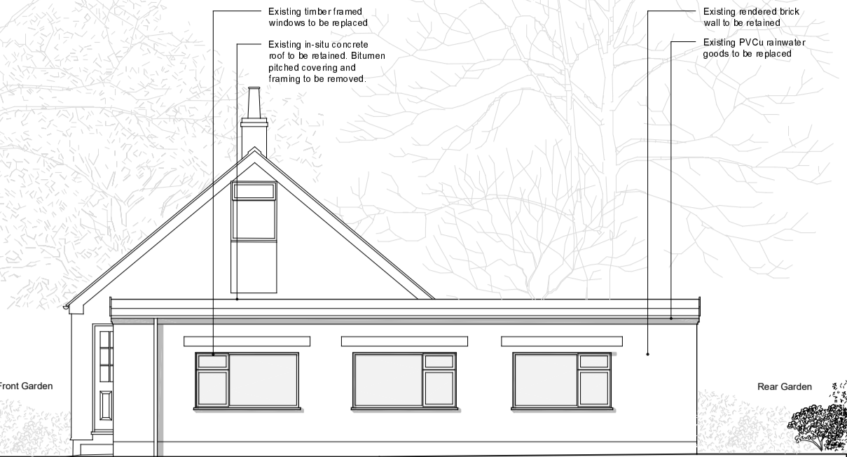
Outbuilding Existing East Elevation 1:100 @ A1
