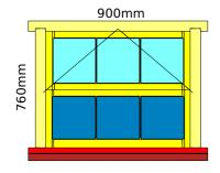
4mm Clear Toughened Float glass (0.25 m2 minimum) 4mm Clear Float (0.2 m2 minimum)
