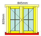
4/4/4 Timbalite low E double glazing, clear float, Krypton gas filled, 1.9 centre pane u-value (0.30 m2 minimum)
