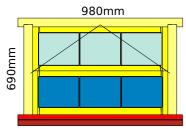
4/4/4 Timbalite low E double glazing, toughened clear float, Krypton gas filled, 1.9 centre pane u-value (0.30 m2 minimum) 4/4/4 Timbalite low E double glazing, clear float, Krypton gas filled, 1.9 centre pane u-value (0.30 m2 minimum)
