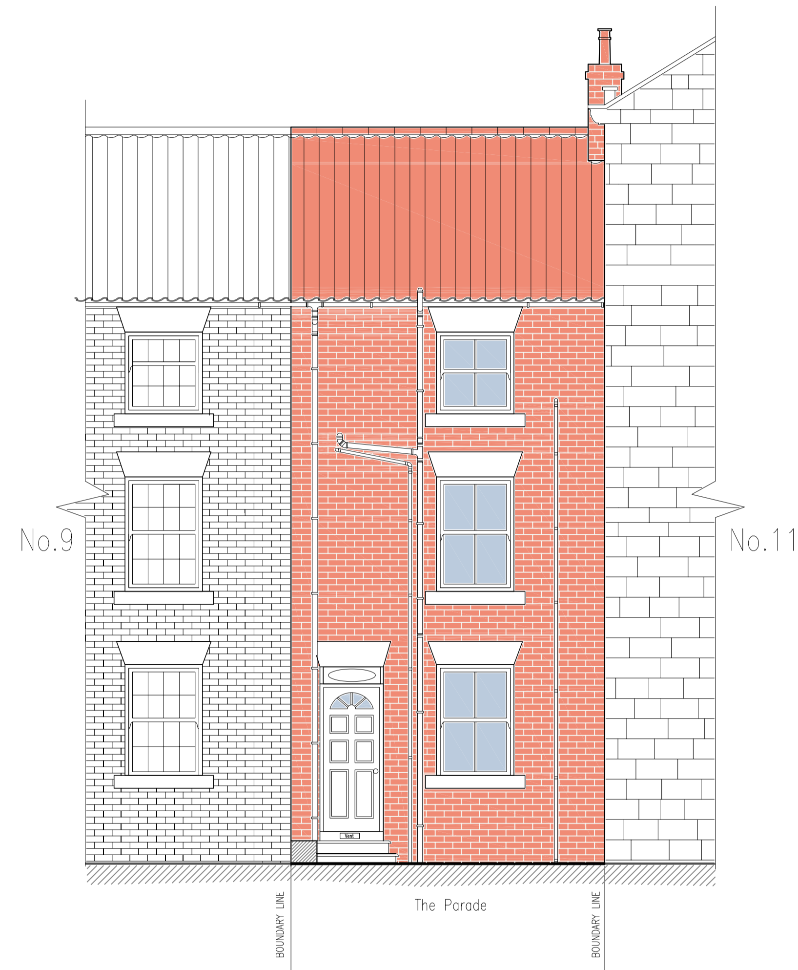
Existing: Front Elevation 1:50 @ A1
