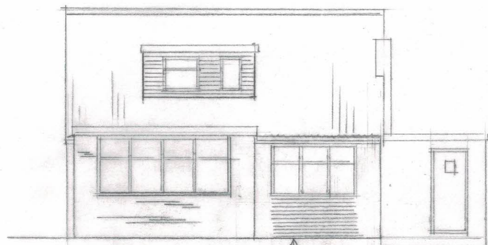
REAR ELEVATION BRICK UP DORMER AND REPLACE WITH UPVC DOUBLE GLAZED WINDOW
