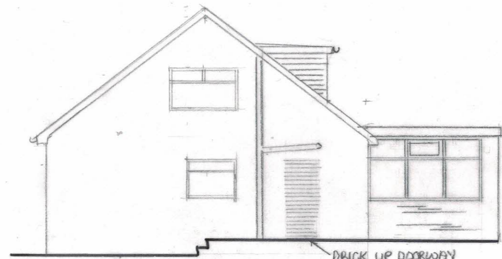
SIDE ELEVATION BRICK UP DOORWAY
