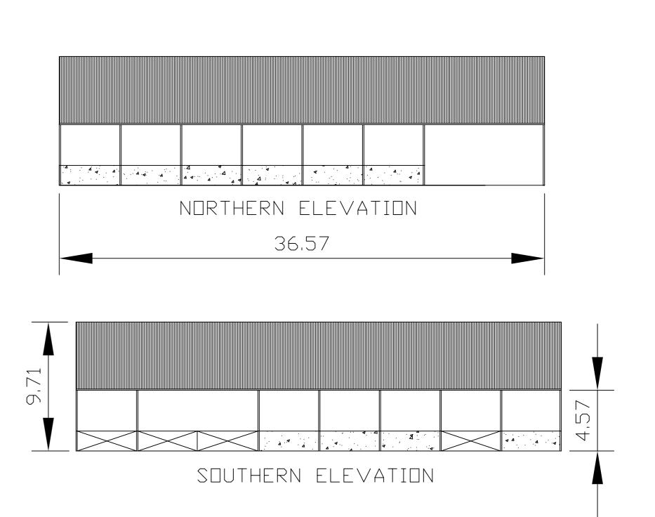
ROOF MATERIAL - FIBRE CEMENT SHEETING GABLE CLADDING - BOX PROFILE SHEETING WALLS - PRE-CAST CONCRETE PANELS FRAME - STEEL PORTAL FRAME
