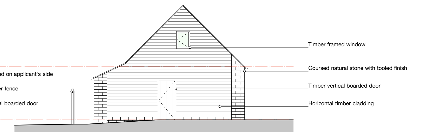
Proposed North Elevation 1:100
