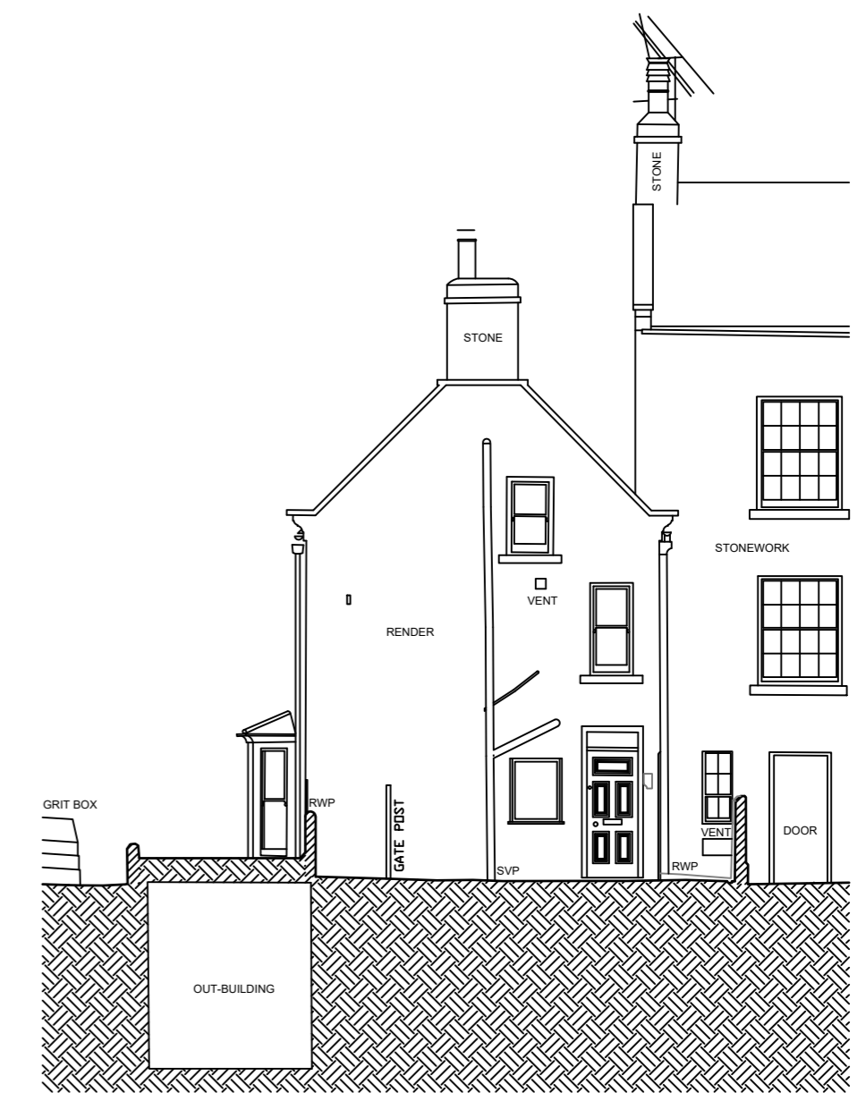
DATUM 4.000m Side Elevation (New Road Elevation)
