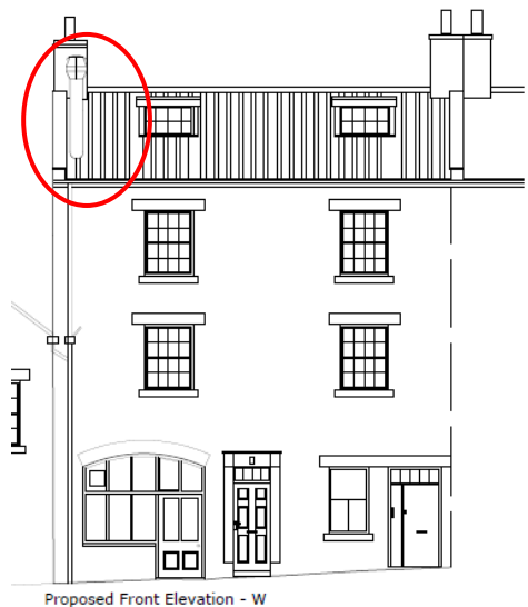
Fig 8. – Proposed flue position against existing stack.
