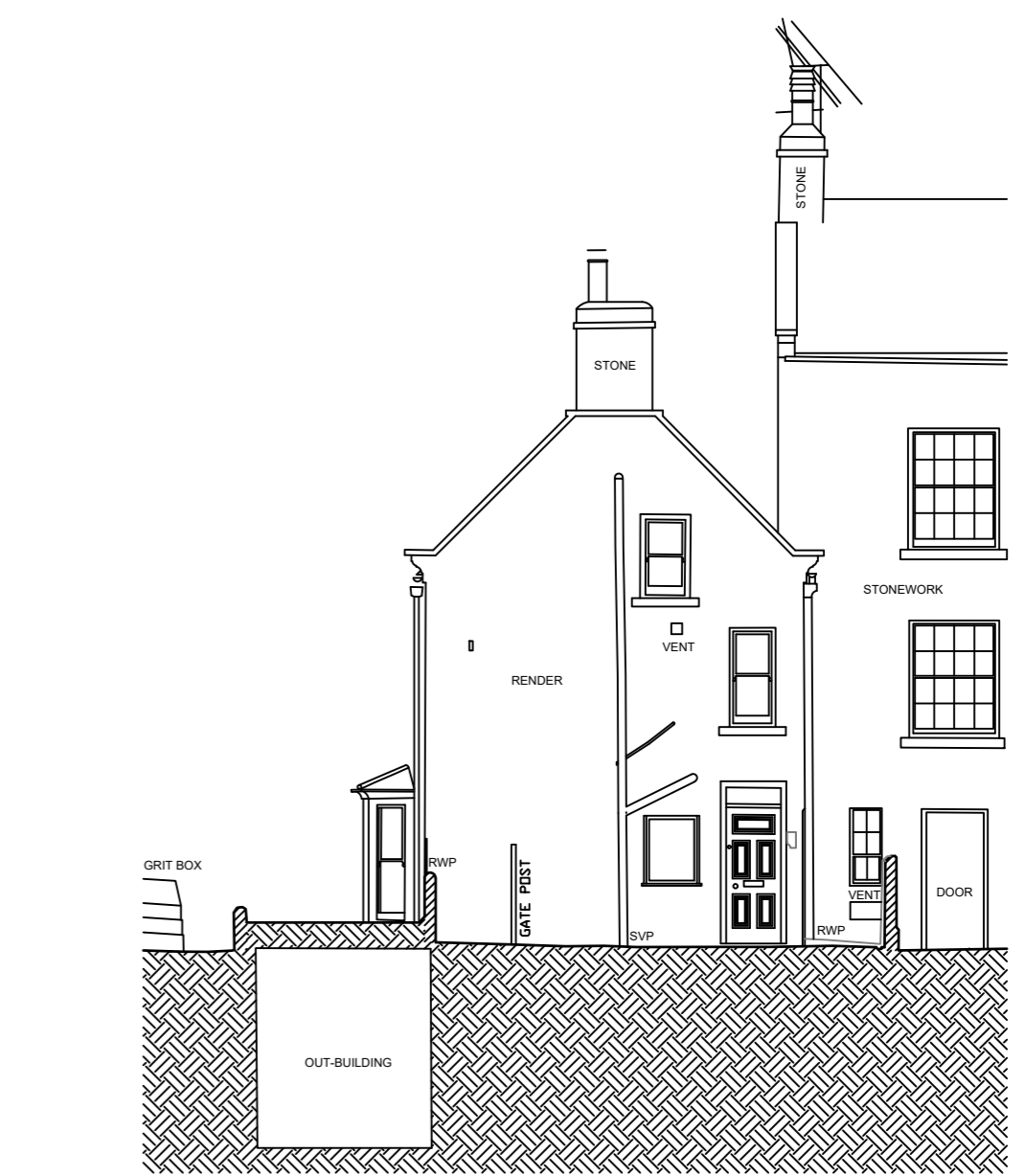
DATUM 4.000m Side Elevation (New Road Elevation)
