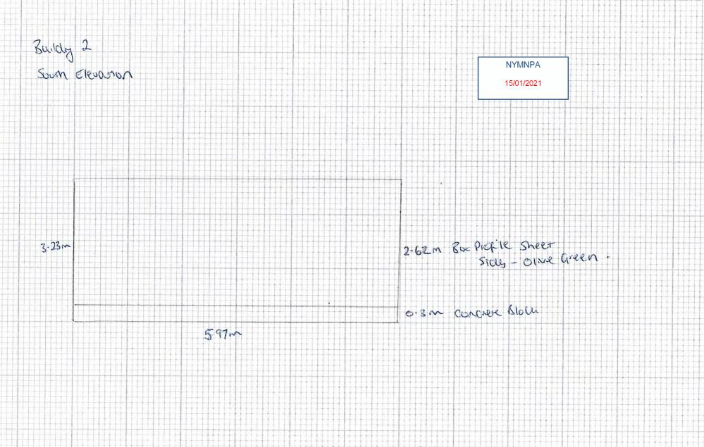
NYMNPA Buildy 2 15/01/2021 West devosion Box Profile Sheet sides - olive areen we wheleves. Existing concrete well.
