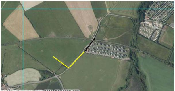
Yellow line marks route of existing OHL to be upgraded. Black line and arrows mark route of extended line and proposed new poles.
