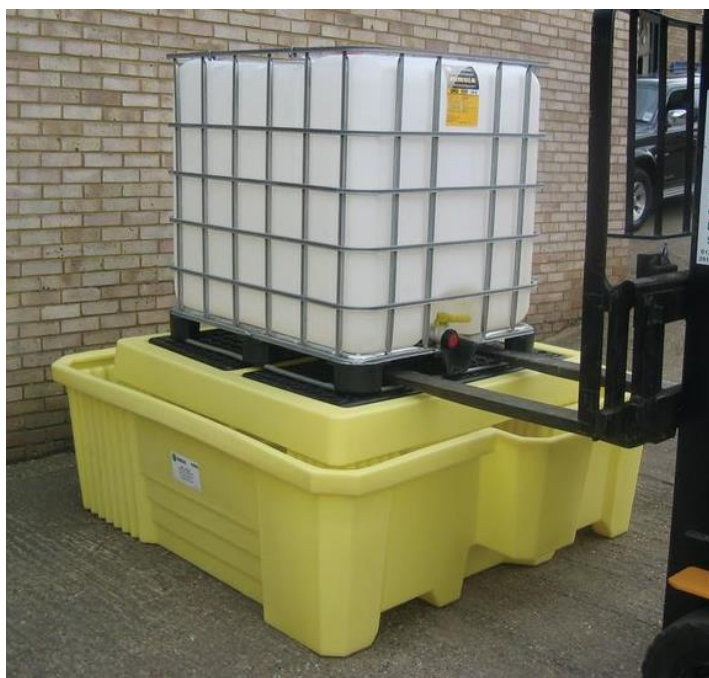
Figure 5: Example of IBC on a bund pallet
