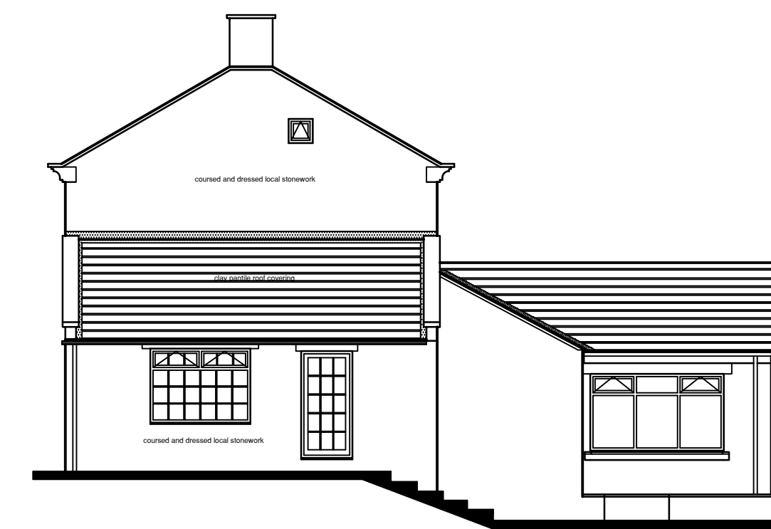
EXISTING SIDE ELEVATION
