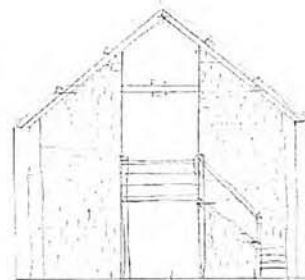
Cross section of building A with open oak staircase from S to N.
