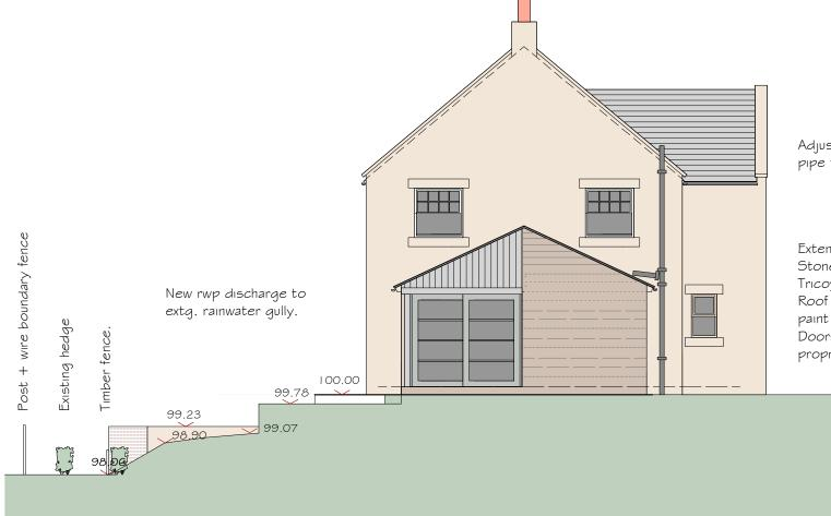
Adjust configuration of soil \$ vent pipe to suit new extension roof.
