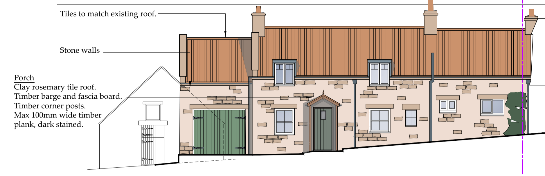
Front Elevation - E Scale 1:50
