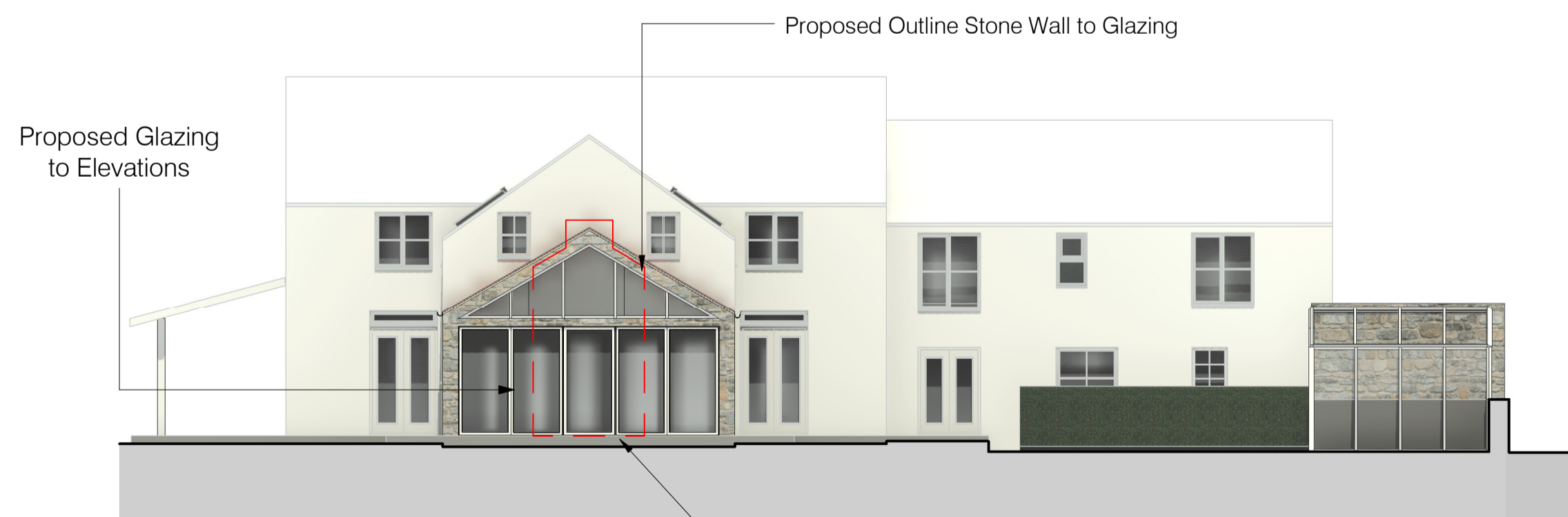
10 Proposed Rear Elevation 1 : 100
