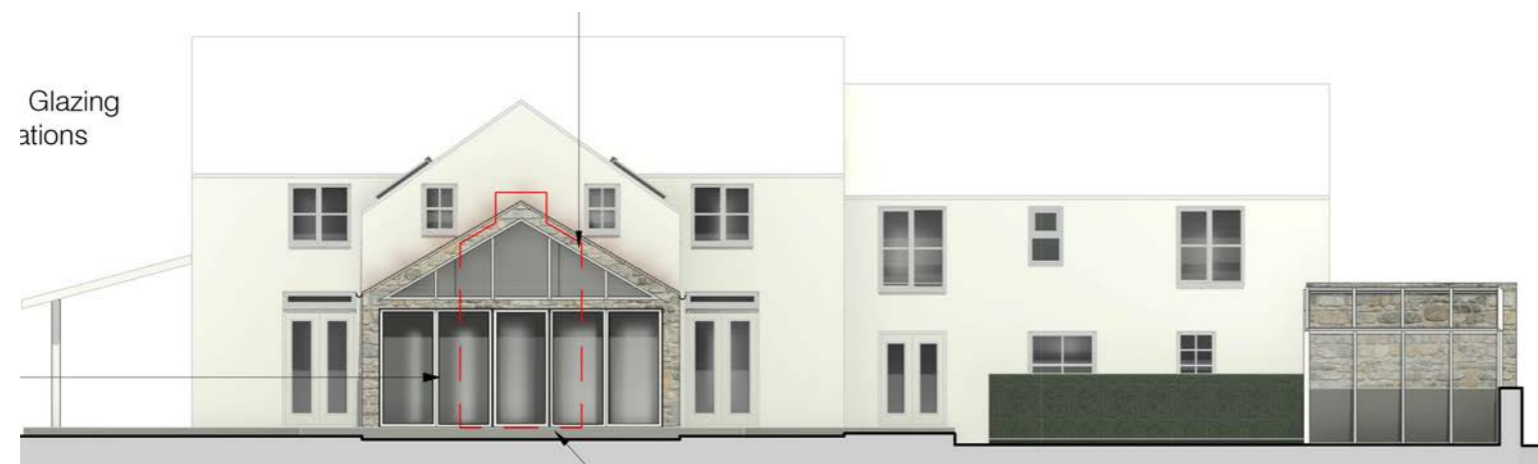
Above is the proposed elevation submitted with this application. Note the existing stone wall corners have been retained and stone walling is shown between the head of the window and underside of roof verge.
