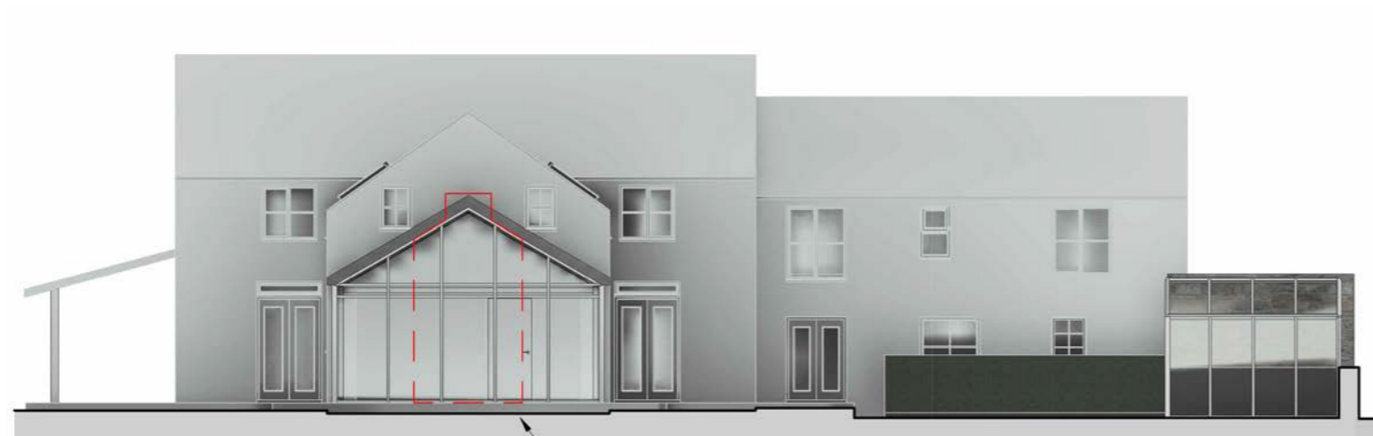
Above is the proposed elevation submitted for pre application advice. The stone wall was removed and replaced by steel columns. The window frame went up to the underside of roof verge.
