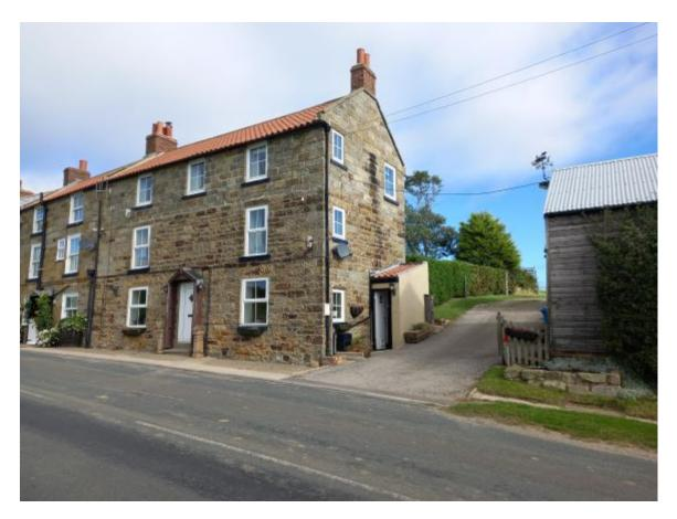
Front and side elevation of Plough Cottage; a three storey end of terrace property of stone under pantile construction. There is an existing single storey mono-pitch porch set well back from the front elevation abutting the shared access drive with a timber clad outbuilding at the other side of the drive.
