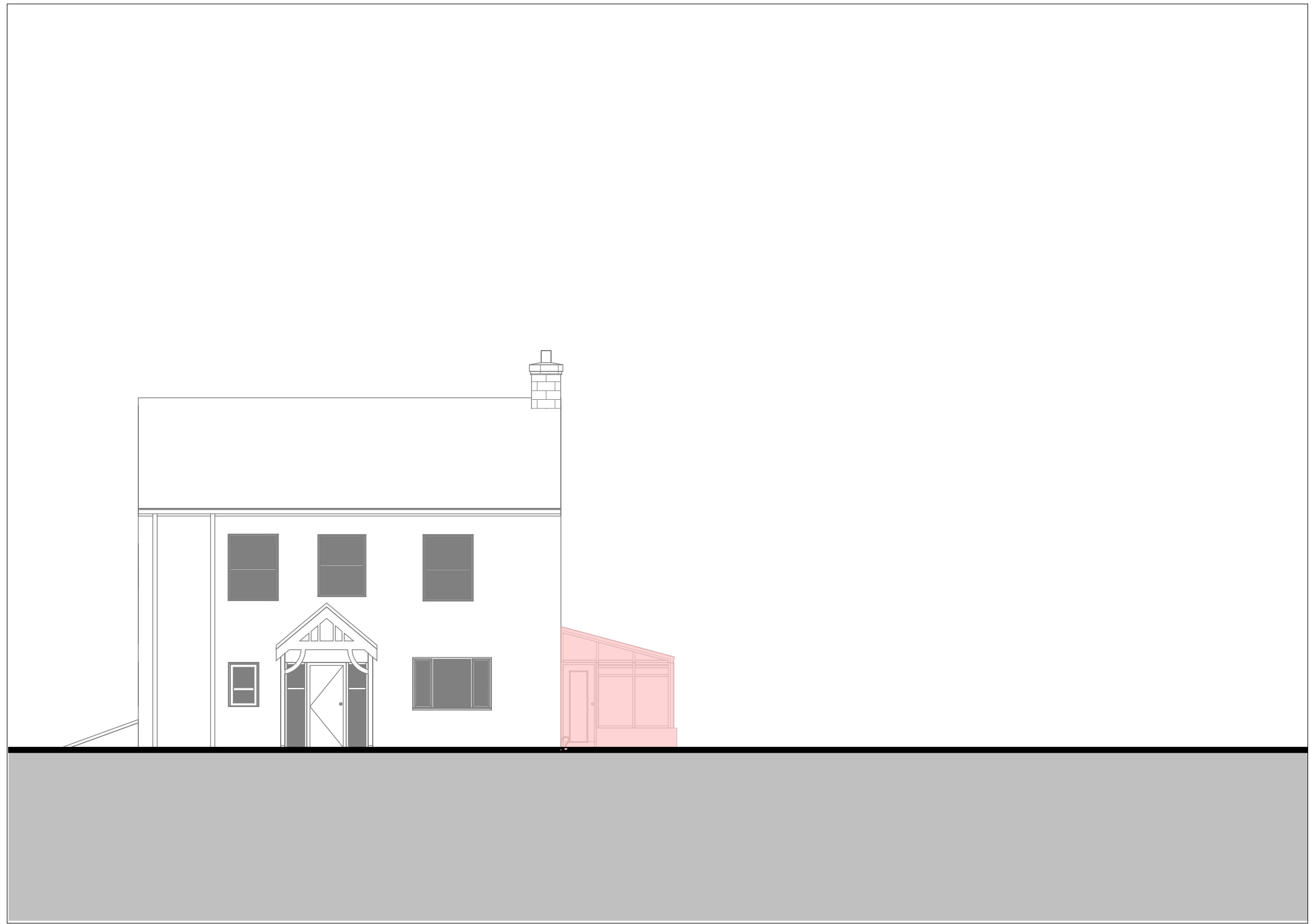
DEF 03-02-DEF - Demolition Elevations - Front 1 : 100
