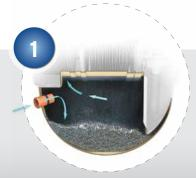
PRIMARY SETTLEMENT TANK Wastewater and sewage flows into the primary settlement tank where the large solids are retained for future removal.
