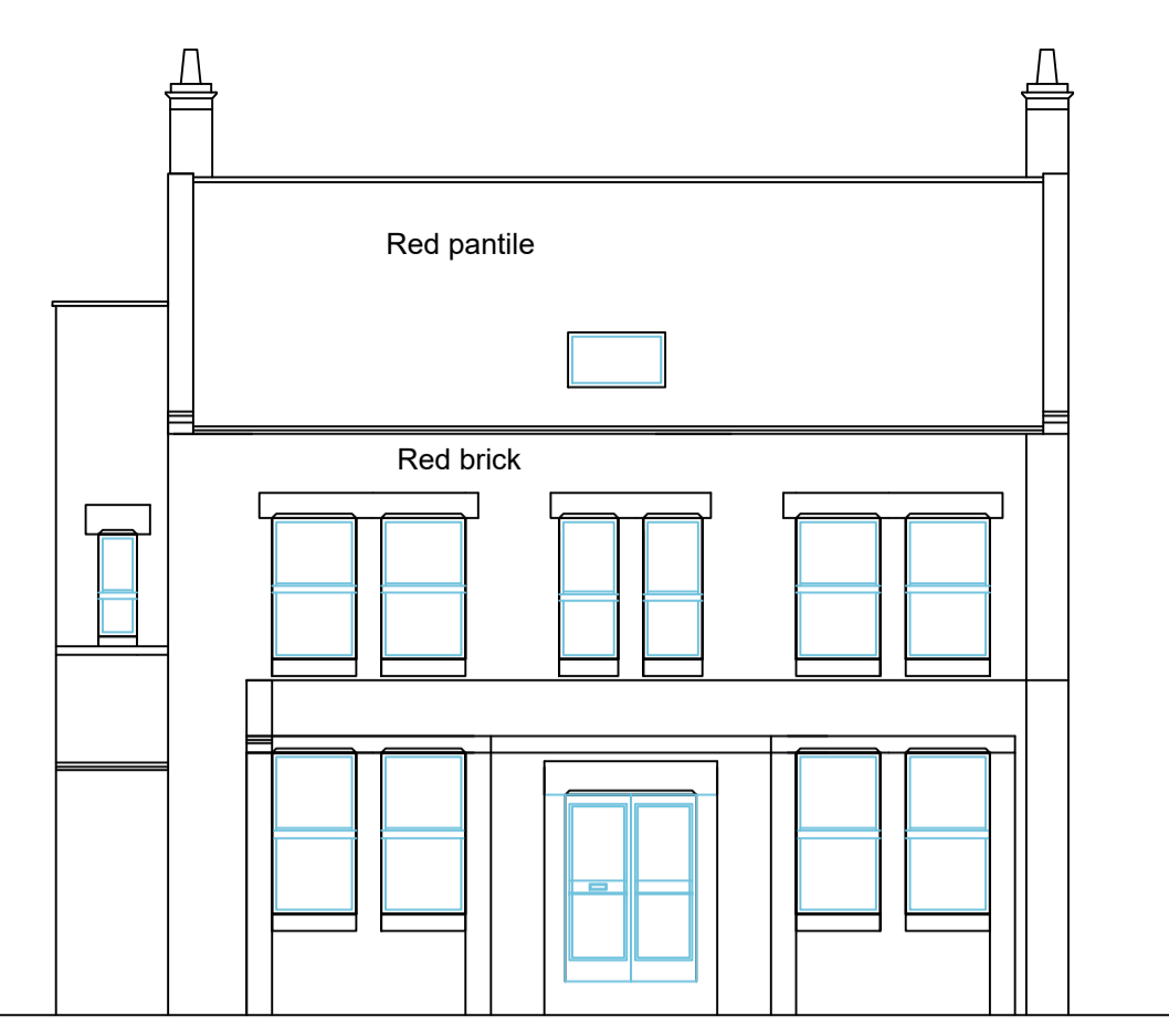
EXISTING NORTH EAST ELEVATION
