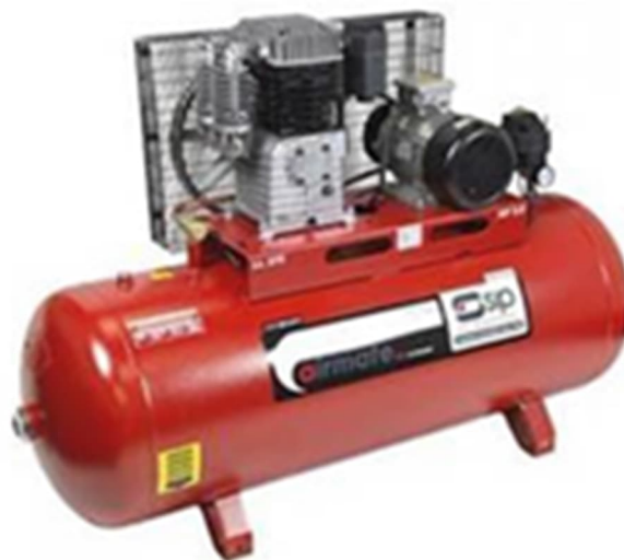
Image 5 – Compressor to service the workshop.
