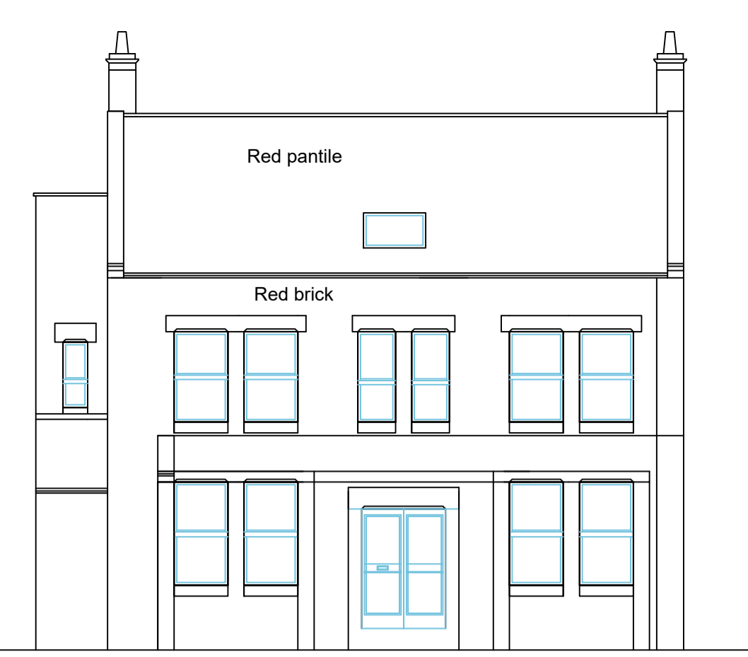
EXISTING NORTH EAST ELEVATION
