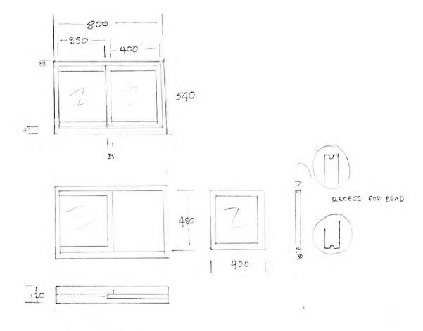
FIXED FRAME + FRAME SCIDING ON A BEAD
