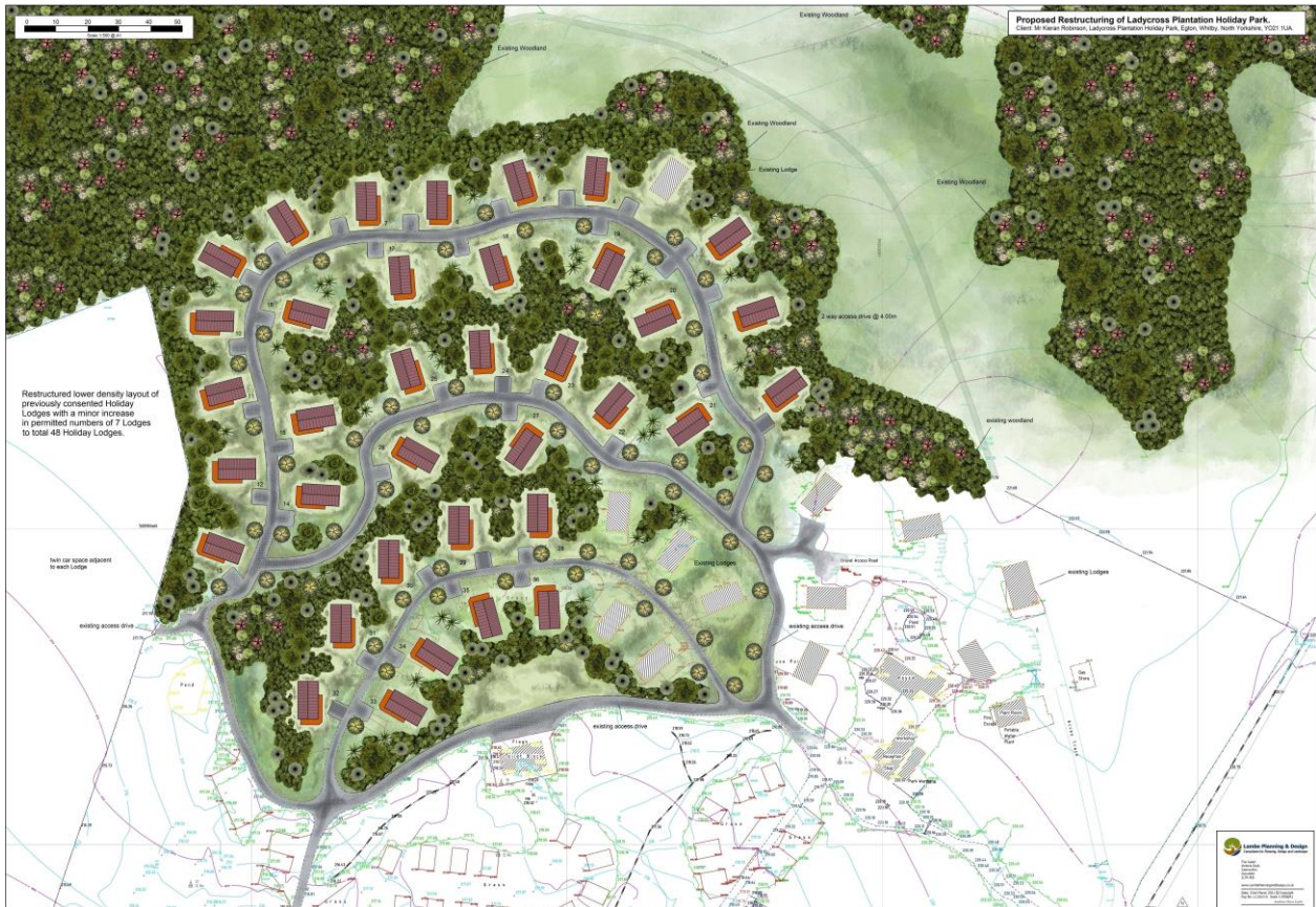
Figure 29. Holiday Lodge Layout Plan illustrating the restructured layout for 36 Holiday Lodges. The plan also illustrates the 12 Lodge locations which have already been sited / implemented.
