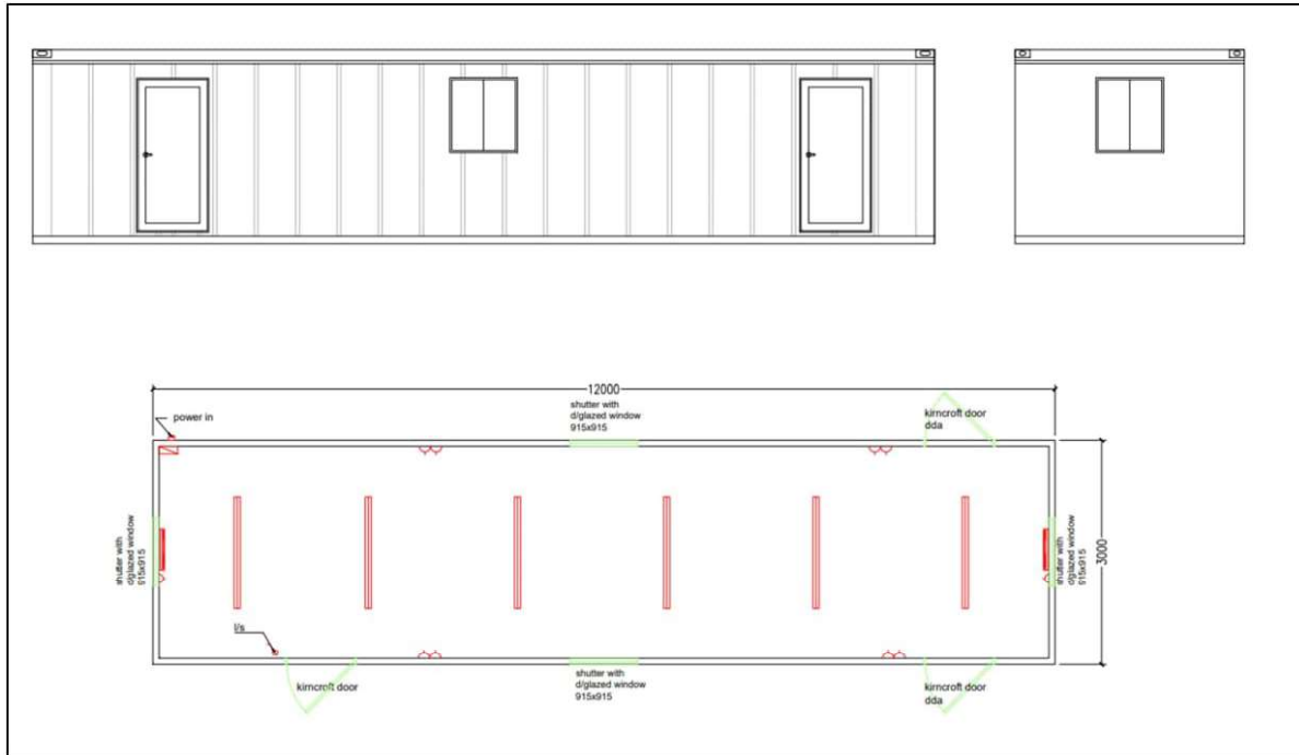
Image 2 – Tally hut dimensions and layout
