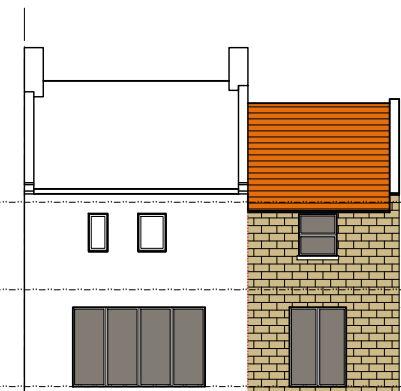
Proposed Rear Elevation Scale 1:100
