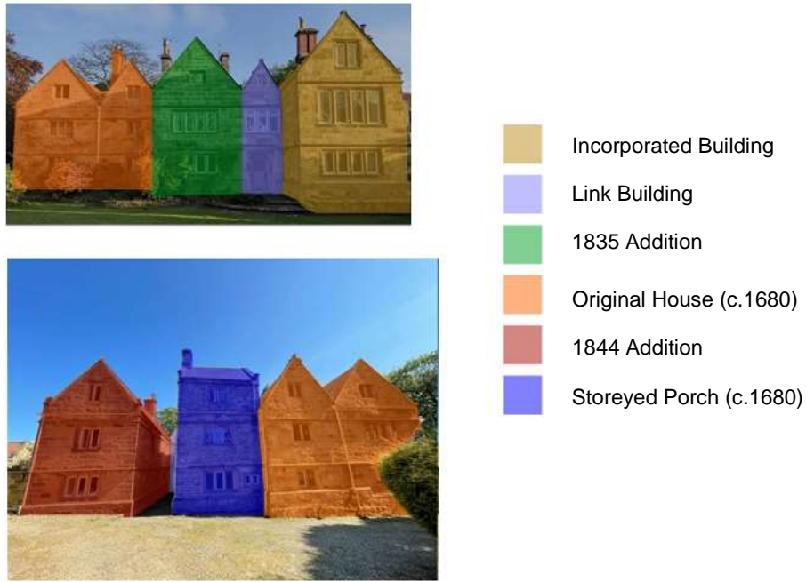
Figure 5 - Historic Plan Progression - ELEVATIONS
