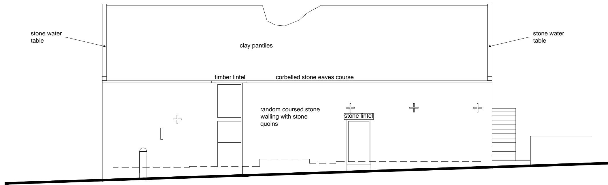
SOUTH WEST ELEVATION
