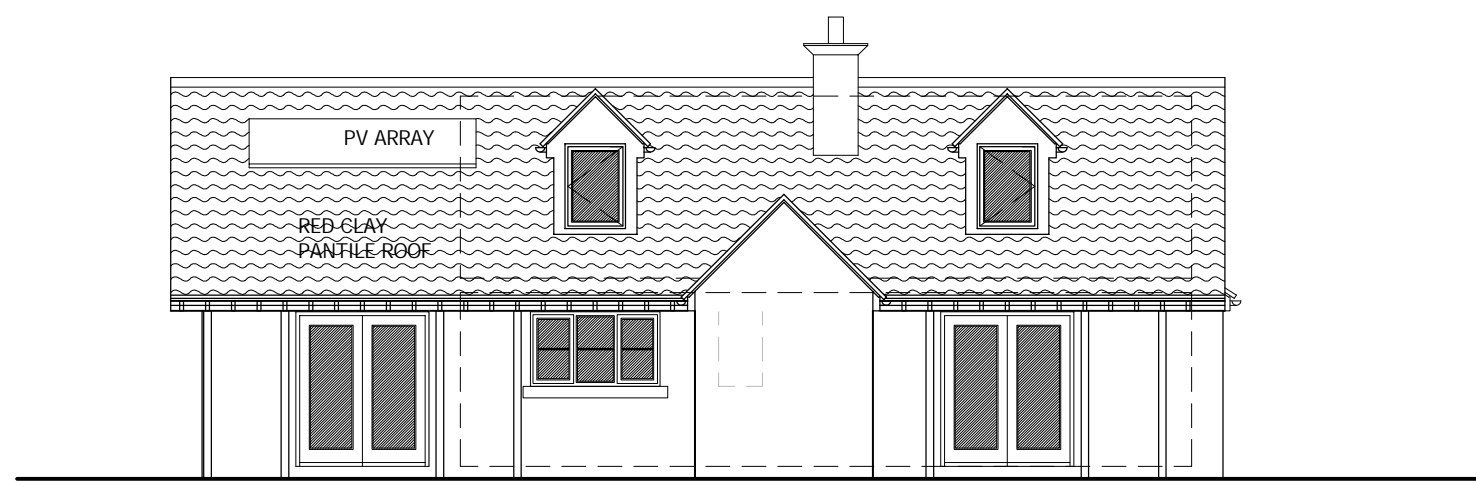
1:100 EXISTING SOUTH ELEVATION
