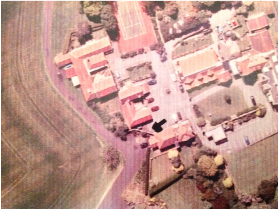
Photo 4 (Above) - This is a photo taken from a 2009 satellite picture of Dunsley. The black mark shows the open path available for surface water to drain away towards a permeable surface.
