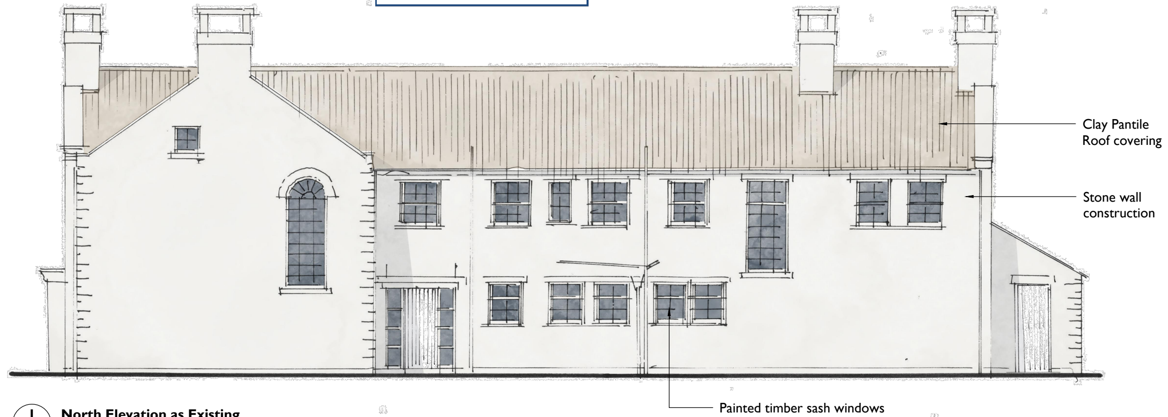
1 North Elevation as Existing 102 1:100
