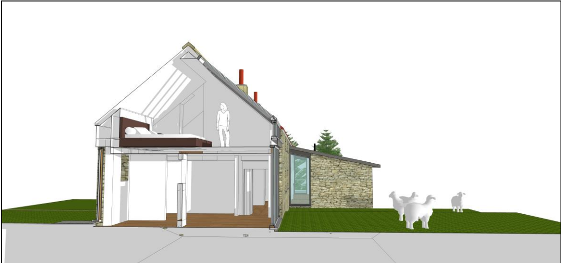
IMAGE 7: SECTION THROUGH PROPOSED MEZANINE FLOOR TO GUEST COTTAGE
