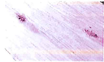
Like most plantation species, pin knots will be found but are not considered defects due to their stability.
