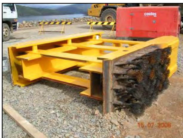
Figure 7: Photos of typical panel joint brush
