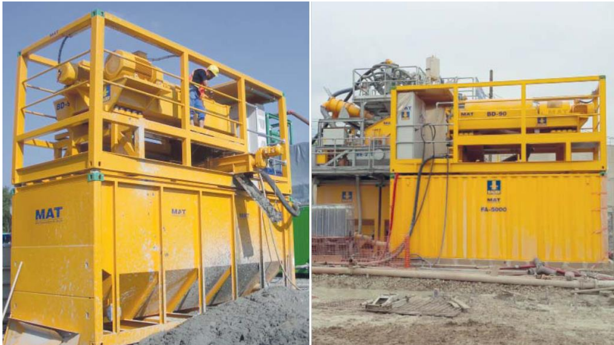
Photograph 8: Flocculant unit (below) and decanter unit (on top)
