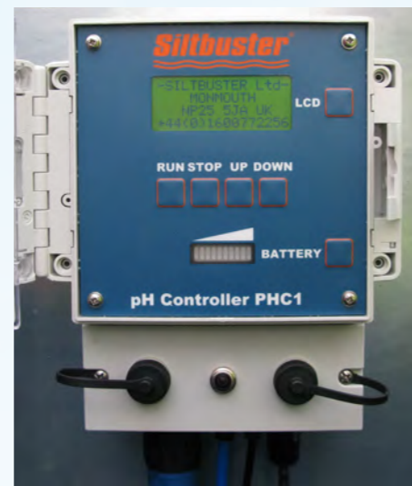
Purpose designed and built pH Controller by Siltbuster for accurate control, recording and neutralising of high pH water
