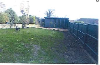
Finally, by comparing photos 5 and 7 you can see that a sleeper edge was placed at the foot of the fence to retain soil which was used to fill the akward gap left at the edge of the deck (Photo 5)) and 'lose the slope down towards the roadside. This soil is 1 sleeper deep at the roadside (225mm) and feathered into the existing levels within 600m of the fenceline.
