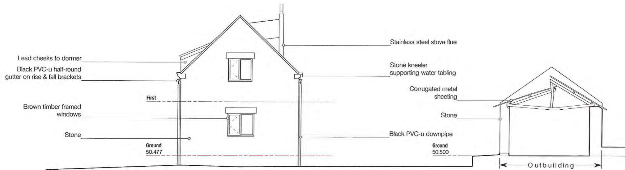
North Sectional Elevation (Side) 1:100
