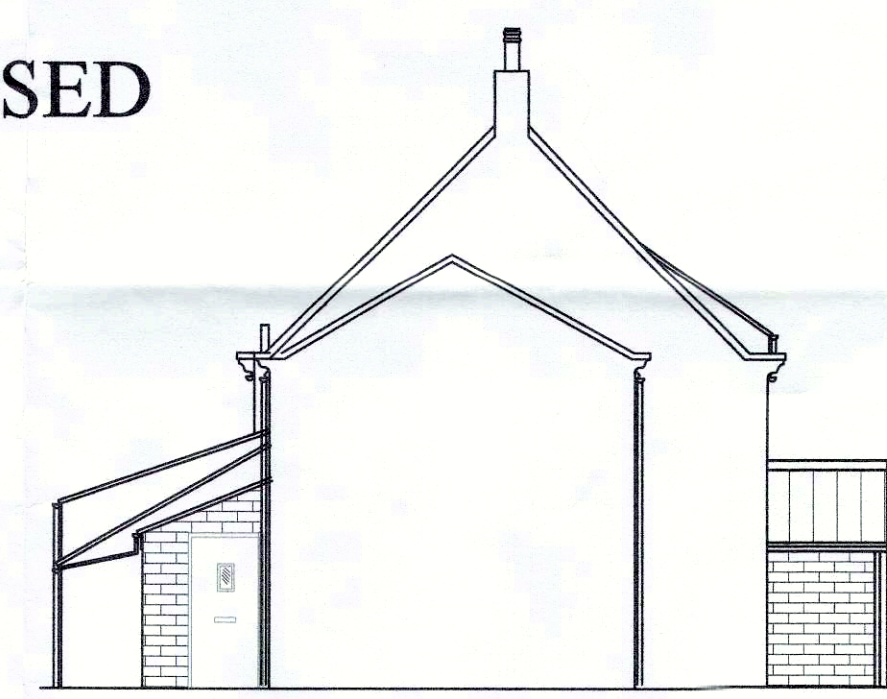
END ELEVATION LOOKING EAST
