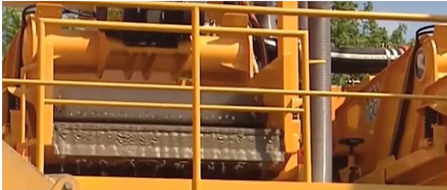
Figure 8 : Desilting equipment separating arisings
