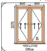
Glazing Includes (31dB) 4T SCoat:20SupAr:4T Low Iron (BLACK SUPER SPACER)
