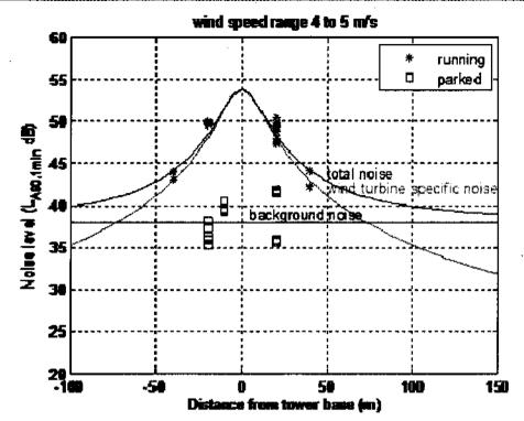
The Iskra Environmental Impact Noise Assessment figures (above) are based on calibrated noise assessments. Modelling is based on using inverse square law calculation which is appropriate for a point source.
