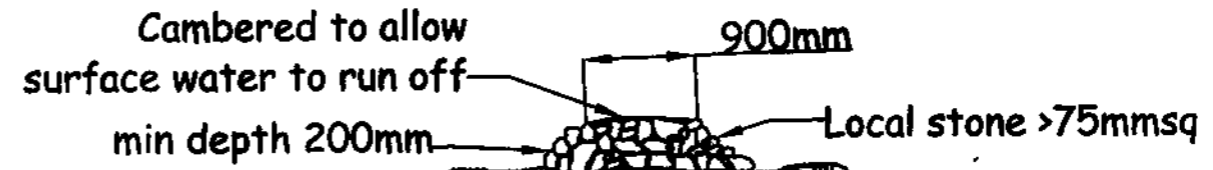
Typical Overtip Detail
