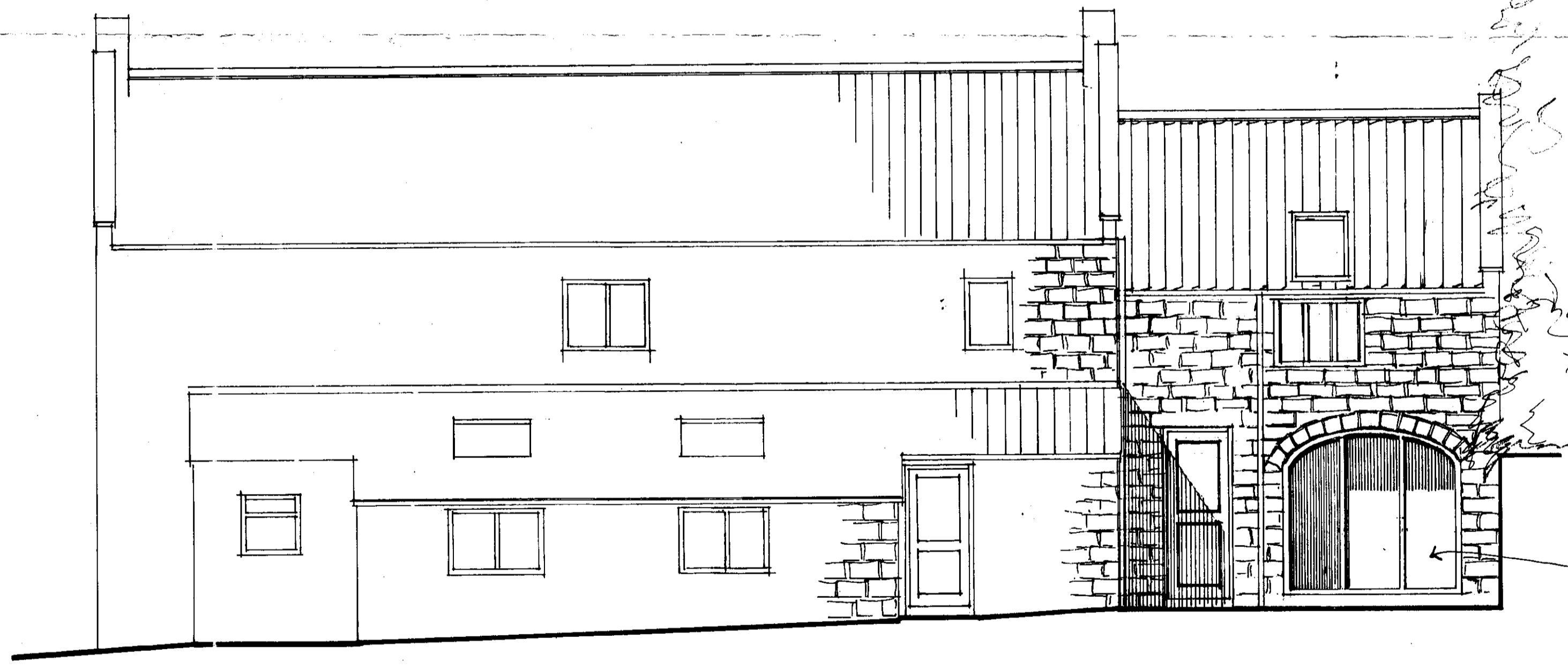
EAST ELEVATION SCALE 1:50
