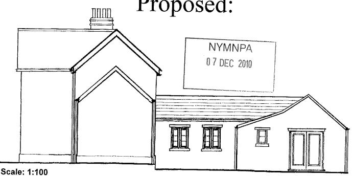
The proposed extension to the side has been reduced from two to single storey. The depth (front to back) of the side extension has also been reduced and the rear wall of the proposed extension now, like the façade of the extension, steps back from the original structure to ensure the detail of the host dwelling is clearly maintained and to ensure the dimensions are in keeping with the dimensions of the original dwelling.
